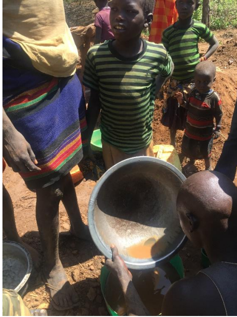
Miner elaborating panning method as an alternative to mercury use in gold extraction
